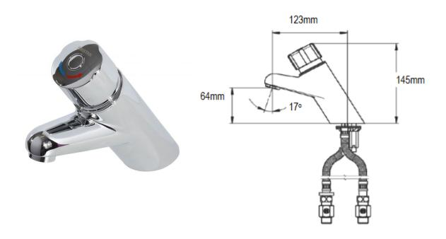
Model TVS6820 is our press button time flow mixer tap. Press button operation to help reduce wasted water. Approximately 15 seconds of flow. Rotate the push button to reduce or increase the water temperature.
